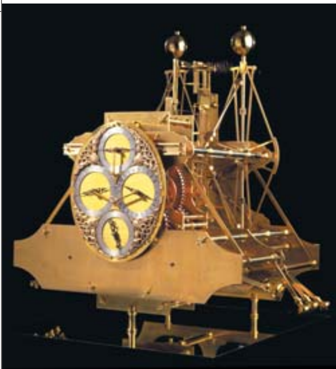
JOHN HARRISON'S H1 sea clock gained its place in history in 1736, when it proved its value in finding longitude on its trial voyage. This replica of the English carpenter's invention was built in 1984.
