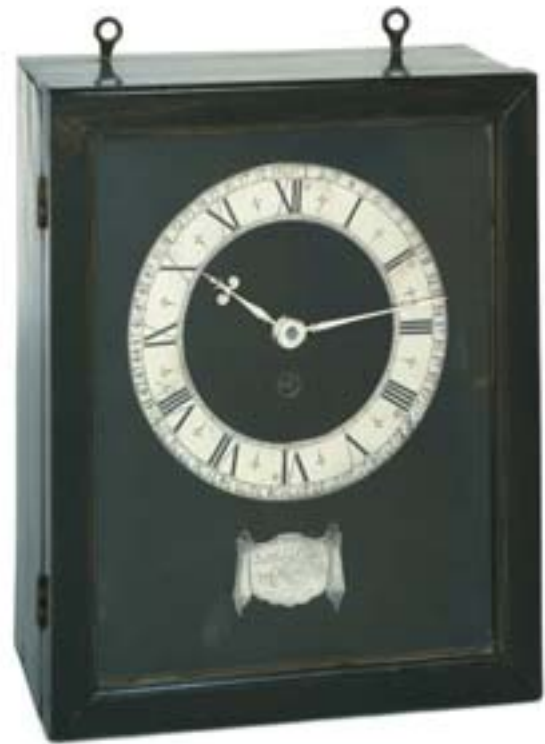
SPRING-DRIVEN MECHANICAL CLOCK was constructed by Dutch clock maker Salomon Coster in 1657. Coster collaborated with Christiaan Huygens, the Dutch scientist who first applied the pendulum to the mechanical clock.
